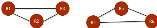
Fig. 3: Relay Connections with two disconnected subgroups of relays, one for each bus in two-bus system.
