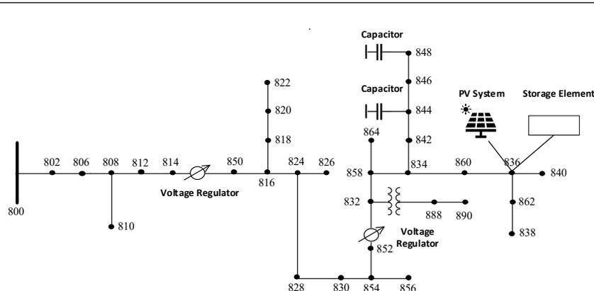
Fig. 1. Electrical distribution network one-line diagram which was based on the IEEE 34 bus test system with PV and energy storage added.
