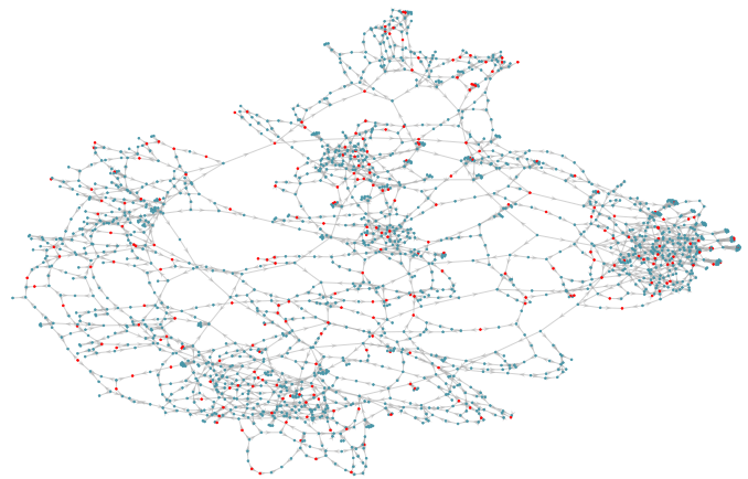
Fig. 1: Graph model of the 2,000-bus power grid of Texas with red nodes indicating the buses connected to CSs.
